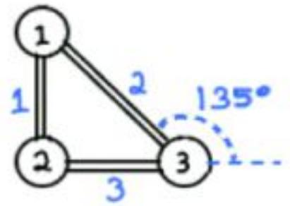
$$A = \begin{bmatrix} \begin{array}{c|c} \text{Node 1} & \\ \hline h & v \\ \hline 0 & 1 \end{array} & \begin{array}{c|c} \text{Node 2} & \\ \hline h & v \\ \hline 0 & -1 \end{array} & \begin{array}{c|c} \text{Node 3} & \\ \hline h & v \\ \hline 0 & 0 \end{array} \\ \hline -\cos 45^\circ & \sin 45^\circ & 0 & 0 & \cos 45^\circ & -\sin 45^\circ \\ \hline 0 & 0 & -1 & 0 & 1 & 0 \end{bmatrix}$$
